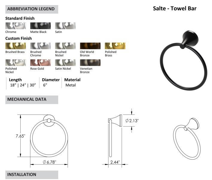
Includes stainless steel screws to install into adequate structural blocking HARDWARE
